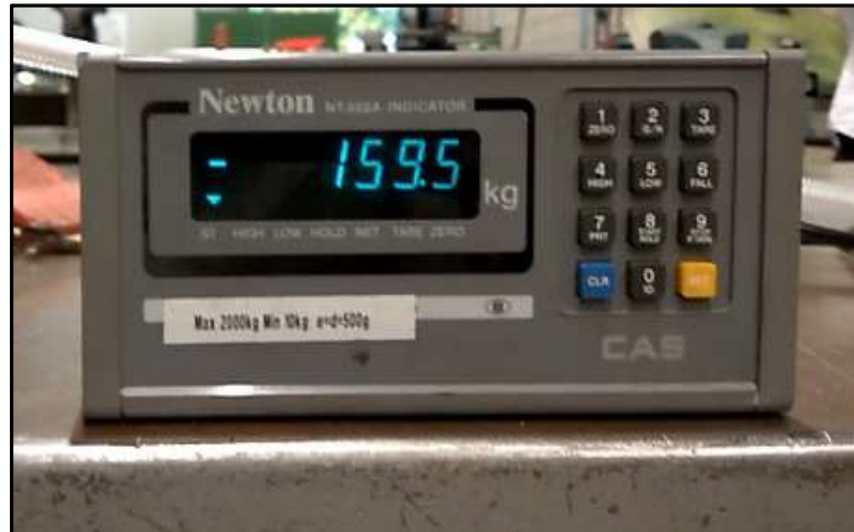
Figure 3: Display of the Load Cell Measurement.
