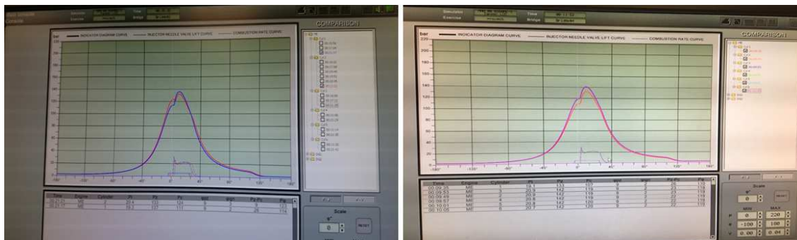
Figure 7: Indicated Power Card with Defect Injector.
