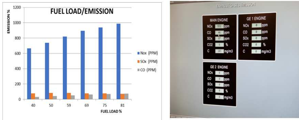
Figure 6: Fuel Load & Exhaust Emissions in Normal Operation.
