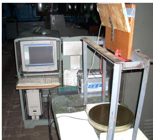
Fig. 1 – The scheme of the installation for defining seed falling time
