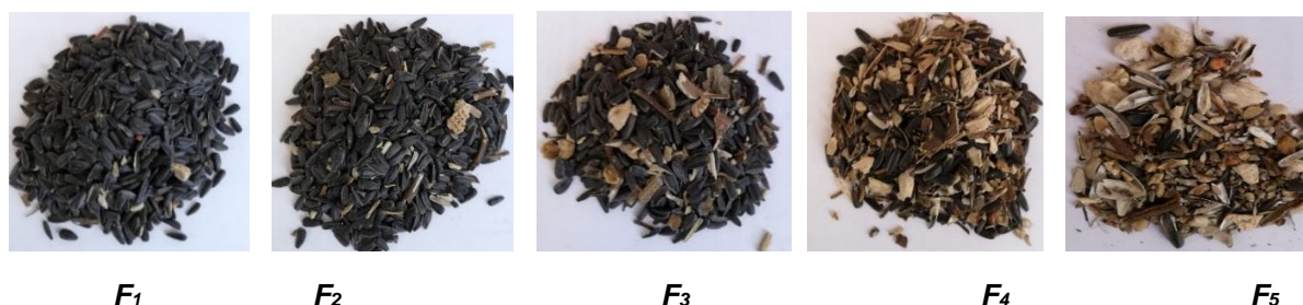
Fig. 6 - Samples collected during sunflower seed conditioning (air flow speed 7.5 m/s)
