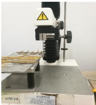
Fig. 3 - Measurement of the rape pod ripping force using a texture analyser
