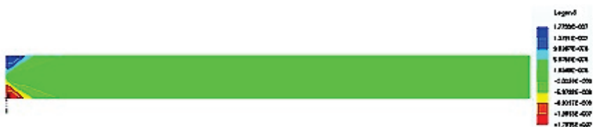
Fig. 16 - Distribution of the equivalent plastic deformation in the perfect elastoplastic matrix.
