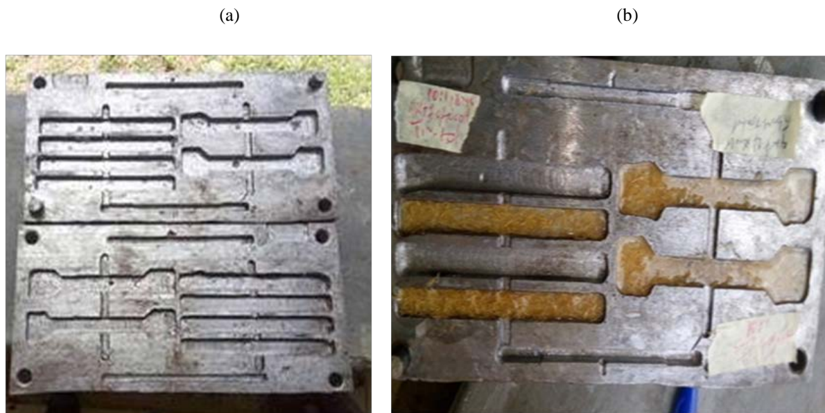
Fig. 1– (a) Fabricated Mild Steel Mold and (b) Mild Steel Molds filled with Polymer Samples.
