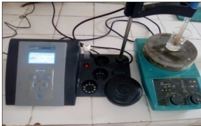
Fig. 18- Apparatus for reading the pH of the acid solution.
