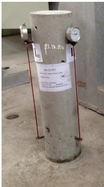
Fig 11. Arranging measuring indicator on specimens without load
