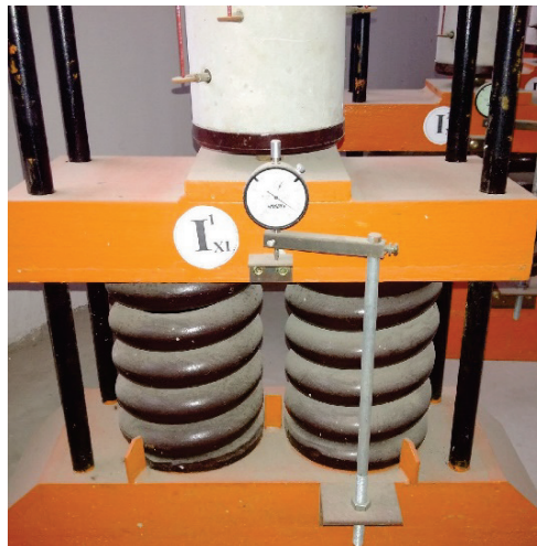
Fig 8. Arrangement of deformation spring indicator
