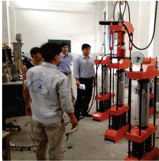
1- Base plate; 2- Spring; 3- Steel bracket bottom; 3a- Steel bracket above; 4- Frame 5- Testing specimen; 6- Lifting jack; 7- Initial frame; 8- Load cell; 9- Indicator a. Detail of the loading system b. Photo of loading system
