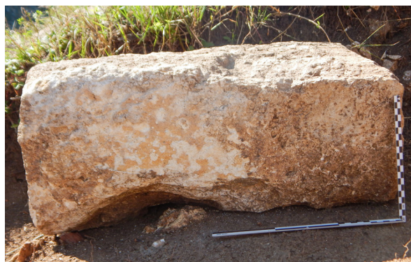
Fig. 5. Boutisse (oolitic limestone block, set perpendicular to the wall surface), from the surface of which the mortar sample was taken (Foto I. V. Ferencz 2016).
