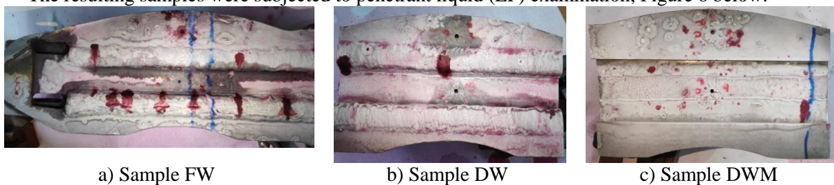
Figure 6. Examination of the samples with penetrating liquids
