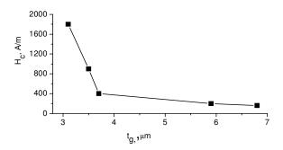
Fig. 2. Dependence of coercivity of MW on the glass cover thickness.
