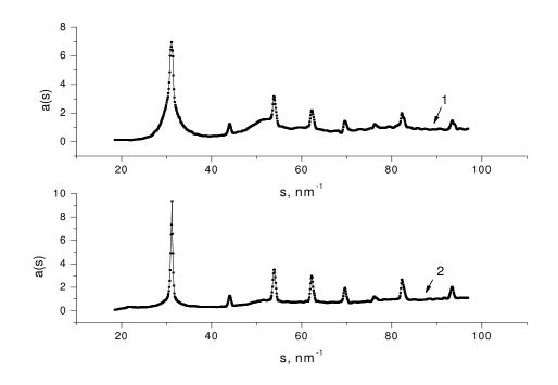
Fig. 1. Structure factors of initial MW: 1 – d/D=0.54, tgl=6.8  $\mu m;$  2 - d/D=0.75, tgl=3.1  $\mu m.$
