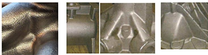
Figure 4. Smooth as cast surface
