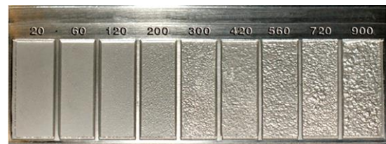
Figure 5. AFS C-9 Micro finish comparator
