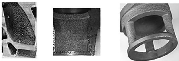
Figure 3. Rough surface inside the casting due to core
