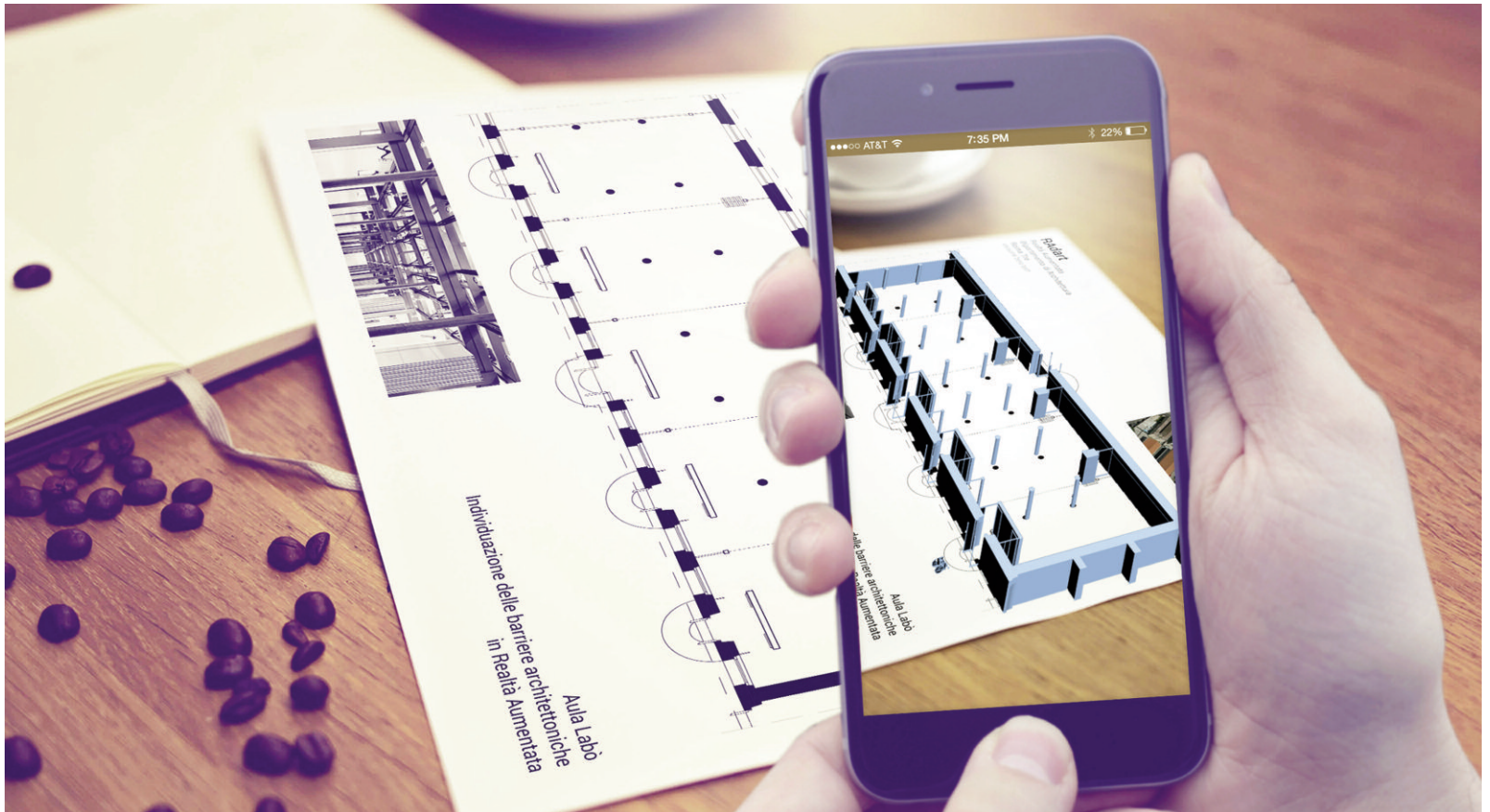
Fig. 9 - RAART application developed within the Department of Architecture of the Roma Tre University. The application recognizes the plant as a marker and associates it with a three-dimensional model with animation of a wheelchair that indicates the path without barriers to follow.
