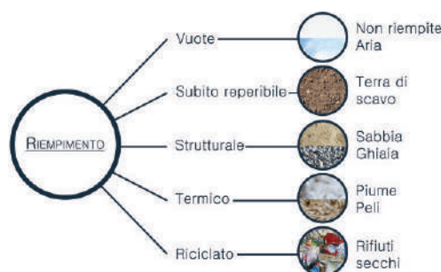
Fig. 8 - Design variables: type of bottle filling.
