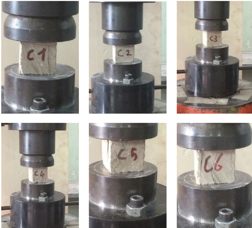
Figg. 21-26 - The samples during compressive strength tests (credits: Scalisi and Sposito, 2017).
