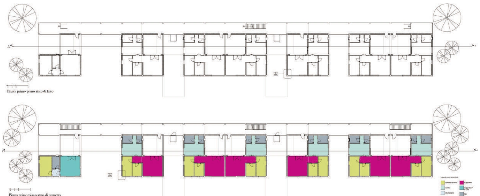
Fig. 5 - First floor plan: comparison between state of art and project from BIM platform (credit: R. Russo).
