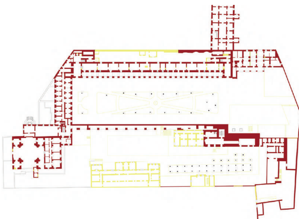
Figg. 5, 6 | SS. Trinità delle Monache Complex: plan of the current state with, in yellow, the expected demolitions; the typological reconfiguration of the monument and the city (credits: R. Capozzi and F. Visconti).
