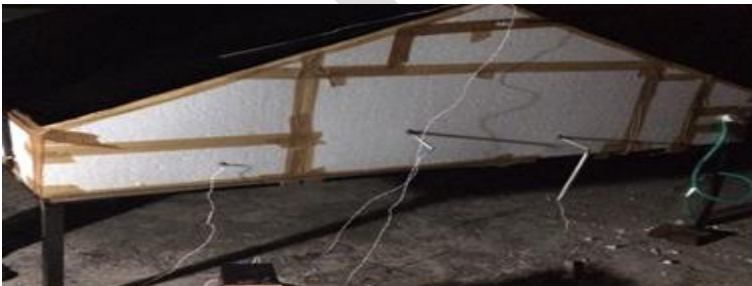
Figure 3: The view of double slope solar still can be seen in figure.
