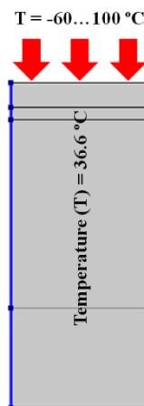
Figure 3 – The initial conditions of heat transfer.
