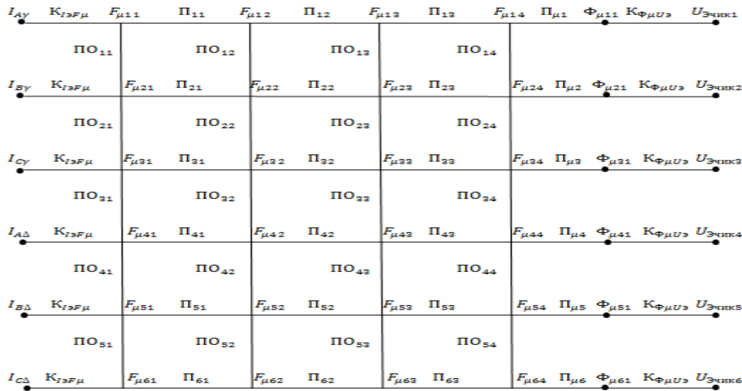
Figure 3. A graphical model that corresponds to the structure of the magnetic part of the sensor for the conversion of primary currents to secondary voltage and reflects the processes taking place in the magnetic switching part.
