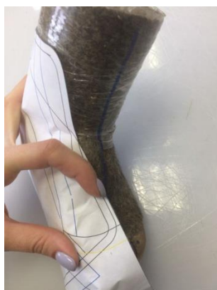
Figure 10 - Position of bonding primer - patterns on the block
