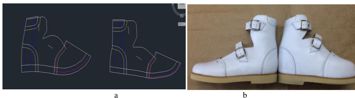
Figure 19 - Drawing (s) and photograph (b) of finished shoes for shortening the limb
