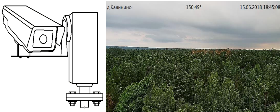
Figure 2. IP-camera on a swivel base mounted on a vertical bracket:
