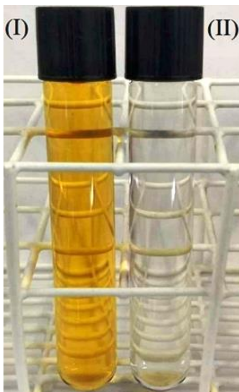
Figure 5. Comparison of bromothymol blue dye color before (I) and after (II) treatment.
