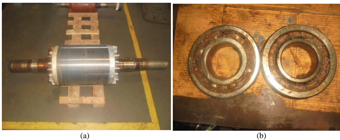
Figure. 18 Parts of 75 kW motor before maintenance: (a) rotor and (b) bearing
