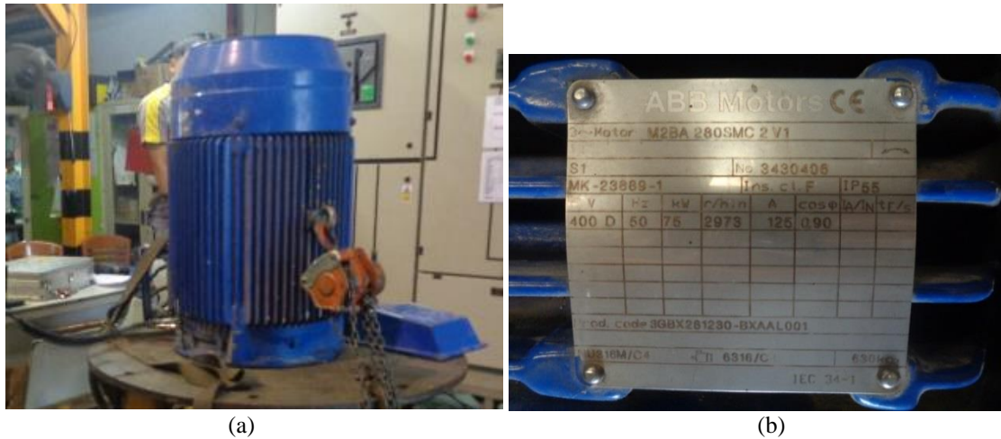
Figure. 16 75kW motor with 2,973 rpm in the experiment: (a) tested motor and (b) motor's nameplate
