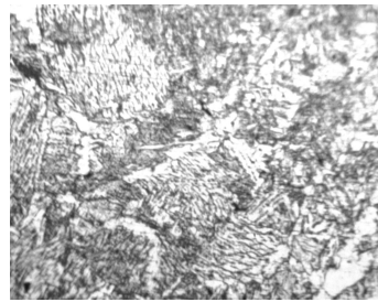
Figure 8. Sample E1T, TIZ, Nital 2%, 100X
