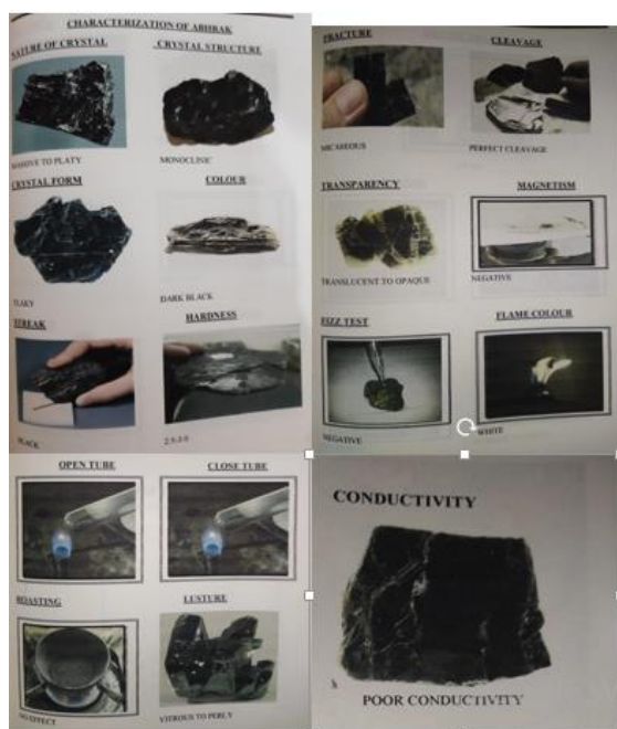
Figure 1 Test conducted for physical properties verification of Abhraka (mica)
