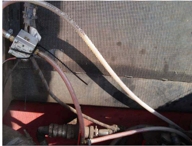
Figure 6. Sensor for volumetric flow mounted in harvester A4000
