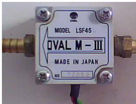
Figure 3. Volumetric sensor to determine the fuel flow
