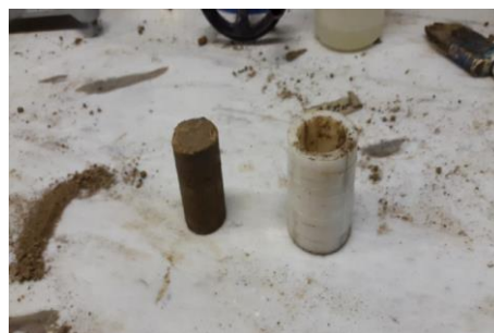
Figure 1. Cylindrical container for single axial compressive test
