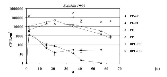
**Fig. 1.** Dynamics of enteropathogen density of the single-species biofilms formed on the PE and PP pipes in inoculated membrane filtered drinking water (PE-mf and PP-mf) or in preexisting multispecies biofilms in inoculated non-sterile water with: **(a)** *E. coli O157*; **(b)** *Y. enterocolitica*; **(c)** *S. dublin*; d – days; HPC of the multispecies biofilms.
