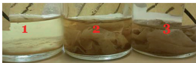
Fig. 3. The triplicate of the tissue microcosms, incubated for 30 months at 25°C and in the presence of Ca(OH) 2 at saturation. Samples 1, 2 and 3 differ in the amount of sediment.
