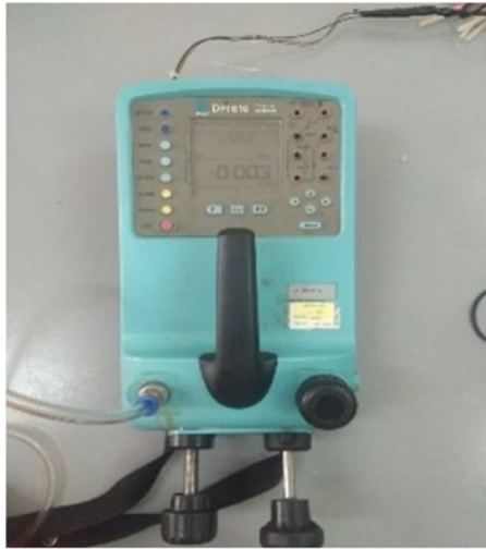
Figure 5. GE Druck DPI 610 calibration device
