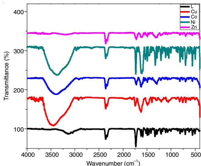
Fig. 2. IR spectra of ligand and its metal(II) complexes
