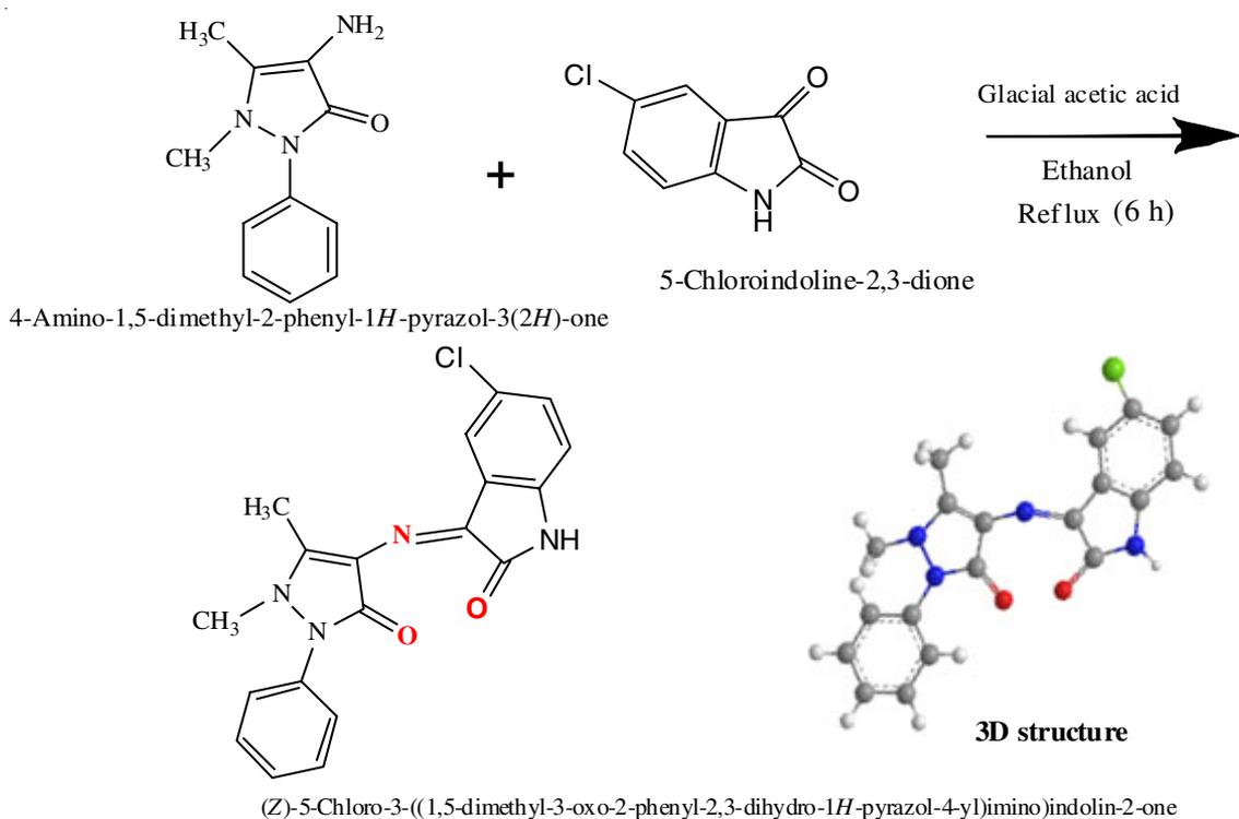
**Scheme-I:** Synthesis of Schiff base ligand (L)
