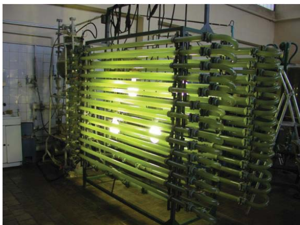
Fig. 2. Experimental tubular photobioreactor of biotechnological complex of the Institute of Hydrobiology of the National Academy of Sciences of Ukraine
