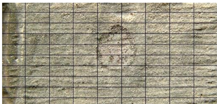
Figure 5. Broken specimen with soldering at x10.5 magnification
