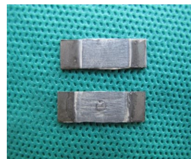
Figure 3. Broken specimens with/without soldering
