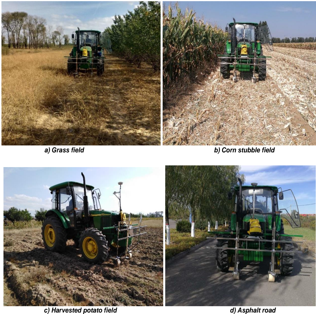
Fig. 2 - Agricultural field and asphalt road profiling measurement
