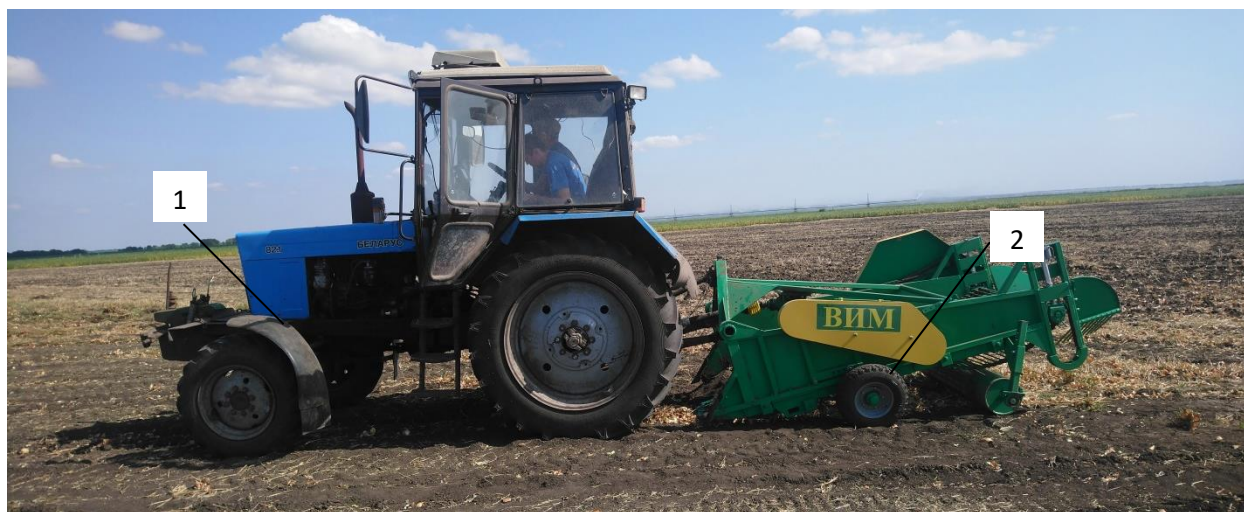
Fig. 3 – General view of the harvester for root crops and onions, equipped with separating rod elevator with an adjustable blade inclination angle and receiving plough share for digging/collecting root crops and bulbs
