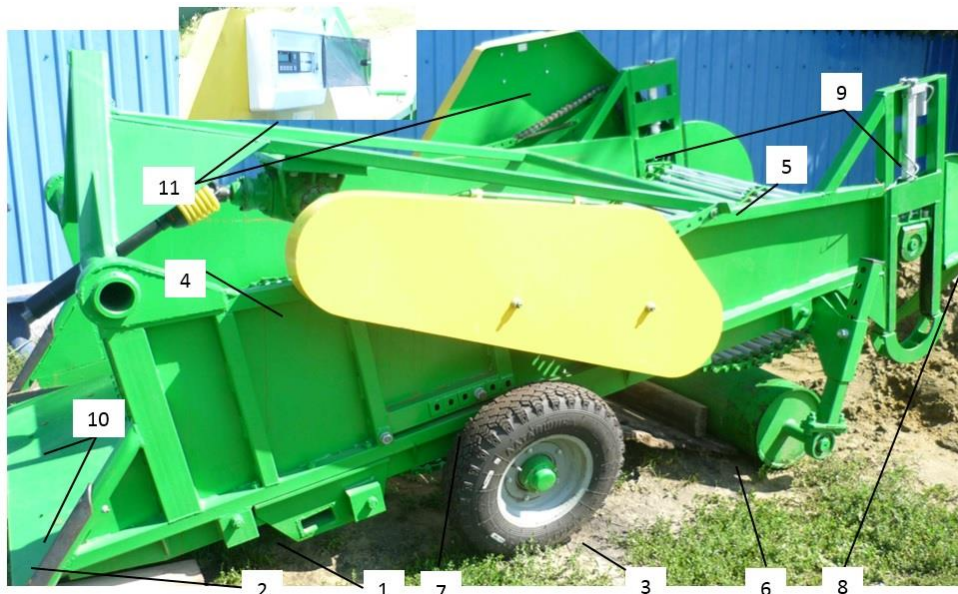
Fig. 2 – General view of the machine for harvesting root crops and onions, equipped with a separating rod elevator with adjustable blade inclination angle and receiving plough share for digging/collecting root crops and bulbs 1 – frame; 2 – receiving plough share for digging/collecting root crops and bulbs; 3 – supporting wheels; 4 – main separating rod elevator; 5 – additional rod elevator; 6 – bed-forming roller; 7 – shaker adjusting plate; 8 – narrowing tray; 9 – electric cylinders; 10 – weight sensor of the digging plough share; 11 – microcontroller
