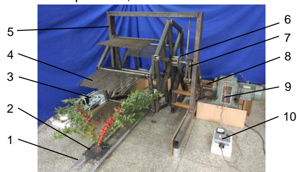
Fig. 2 – Eccentric swing combing mechanism
