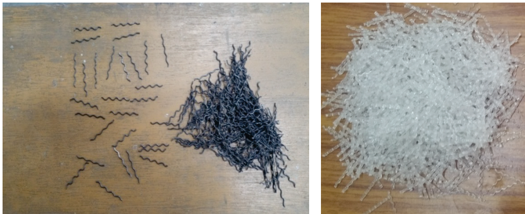
Fig. 2 - Steel Fibers and Polypropylene Fibers used in HyFRSCC.
