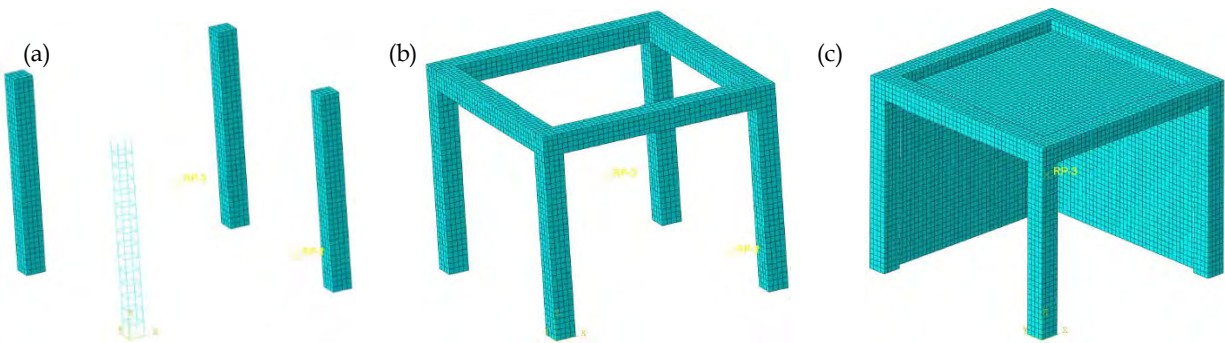
Fig. 2 - Building (a) columns with reinforcement (b) concrete frame and (c) frame with walls and roof slab
