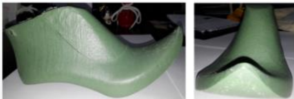
Fig. 5. Pictures reflecting the 3D projection process of shaping the toe of the last and the final mockup of it.
