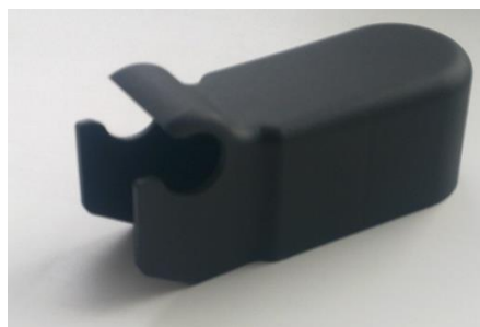
Figure 1 – General view of the wiper arm cap for the cars of "UralAZ".
