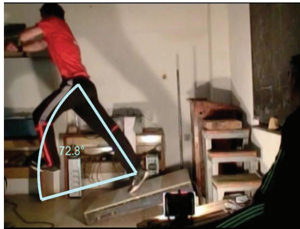
Figure 3. Illustration of the “angle of push back” in the drop jump on an inclined platform
