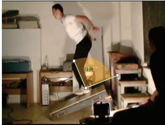
Figure 1. Illustration of the „angle of placing” in the drop jump on an inclined platform
