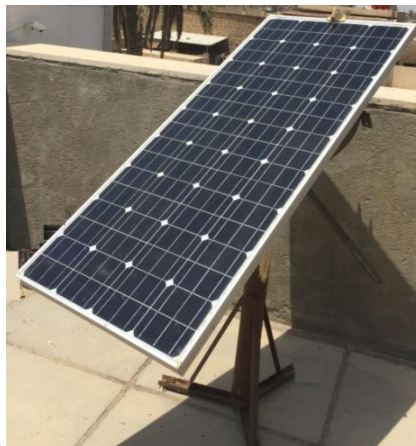
Figure 11: Solar panel equipped with a single axis tracker
