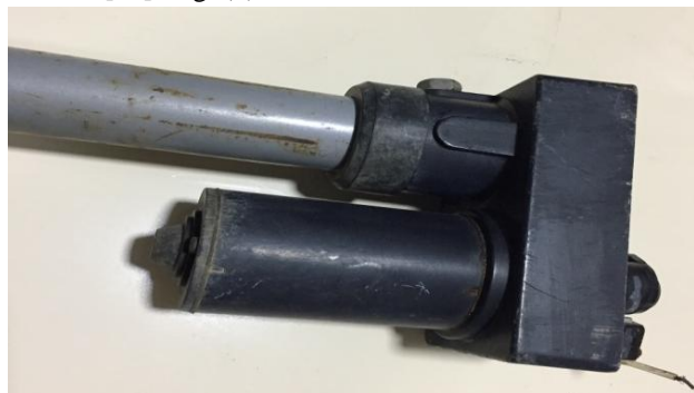
Figure 9: The small 12V, DC motor
