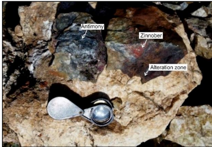
Figure 4: Stibnite ( Sb_2S_3 ) and cinnabar ( HgS ) were identified as ore minerals in the ore samples.
