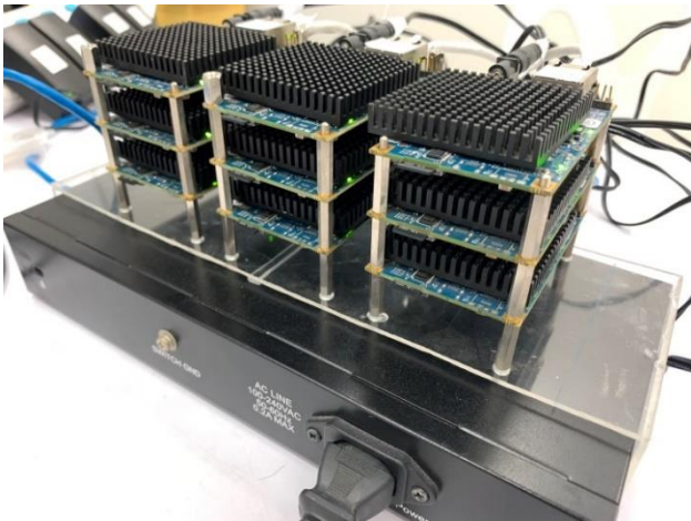
Figure.7 The HDES hardware setup
