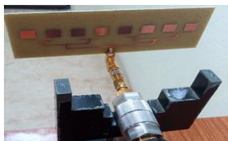
Figure. 19 Eight element microstrip array with full ground plane
