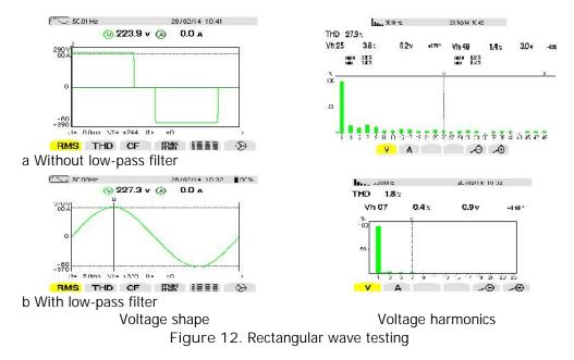
Without low-pass filter for rectangular wave inverter, the boiler worked with interruptions, requiring restart. Add low-pass filter to the boiler is working well.
