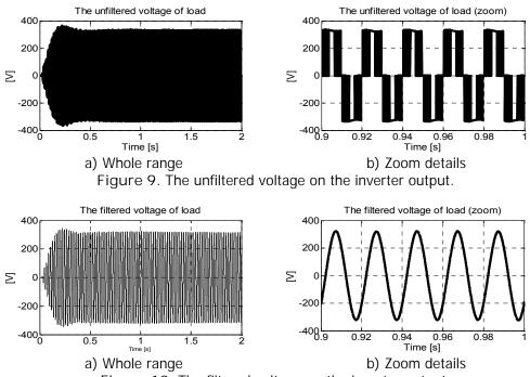
Figure 10. The filtered voltage on the inverter output.
