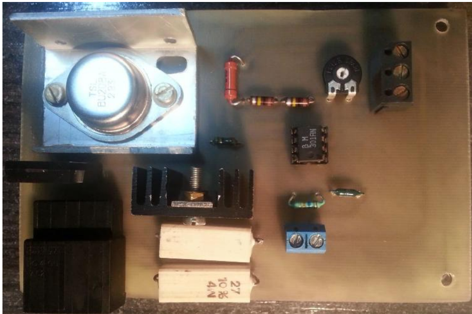
Figure 4. PCB of the braking circuit.
