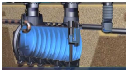
a) Polluted rainwater entrance into the separator
